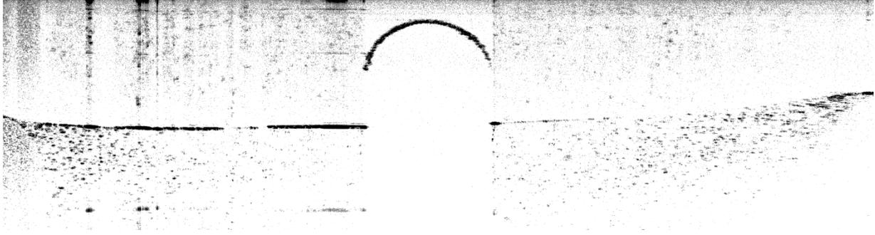
Figure 2. OCT image of microbead on the top surface of an agarose phantom. Image dimensions are 7 mm × 2 mm (width × height).
