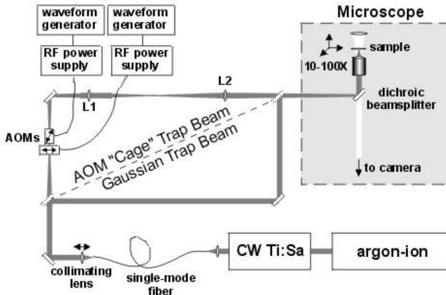
Figure 1: Schematic of the optical trapping setup (not to scale). The Gaussian trap can be accessed by inserting two mirrors on flipper mounts. The lenses L1 and L2 have focal lengths 250mm and 300mm, respectively.
