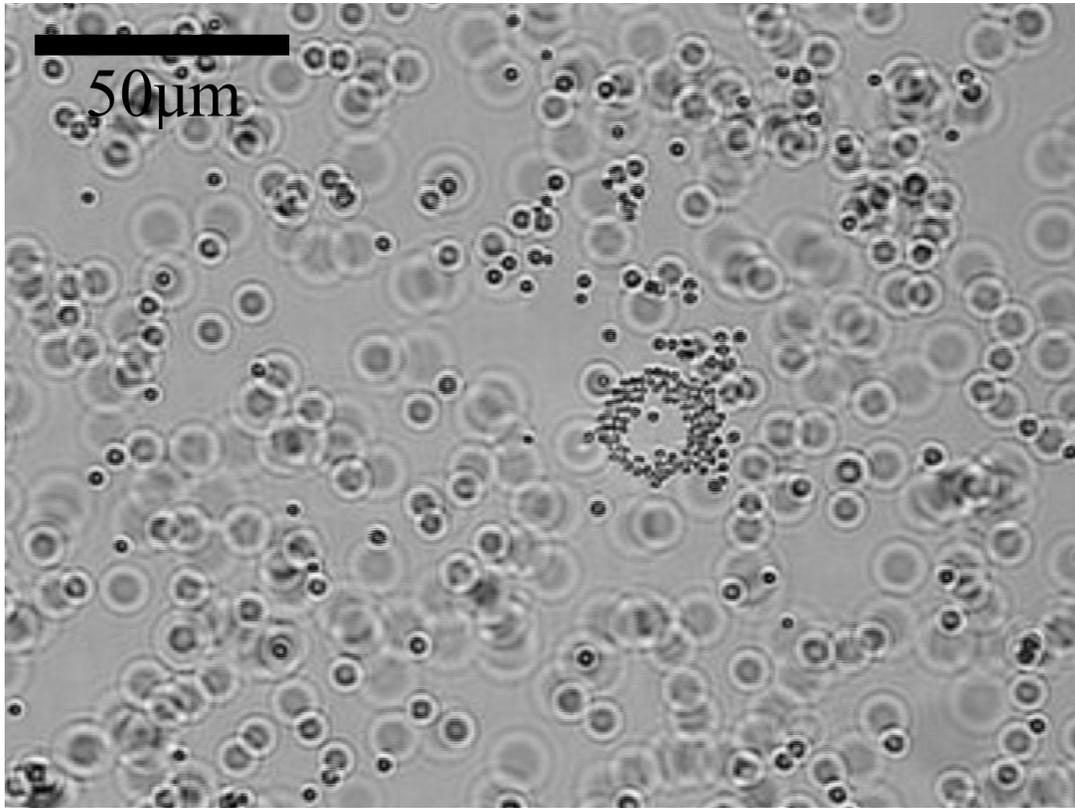
Figure 2: Intensity map of the AOM-based optical trap using  $1\mu\text{m}$  latex beads as an indicator.
