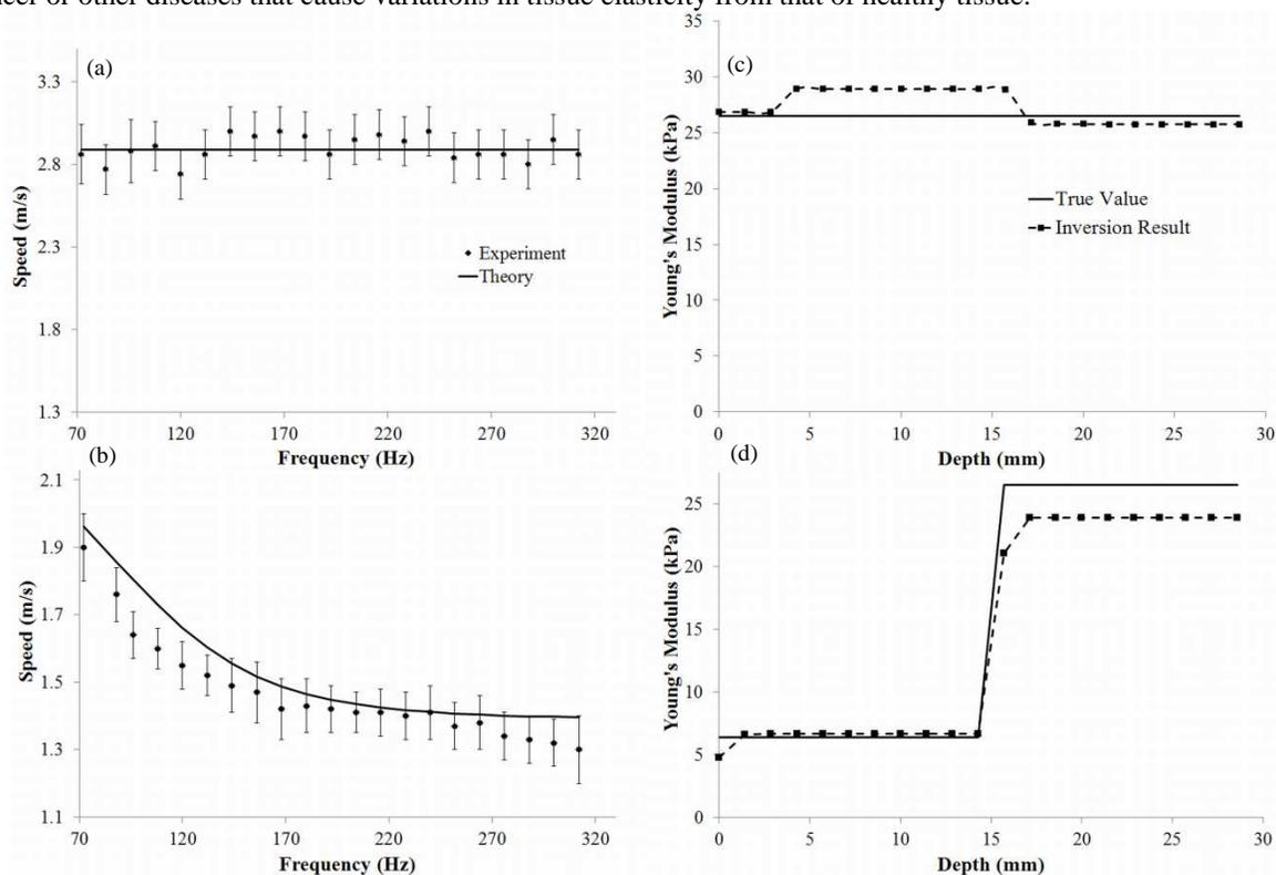
Fig. 2 SAW dispersion curves for (a) homogeneous phantom (b) 2-layer heterogeneous phantom. Also shown is the corresponding Young's modulus profile, obtained by inversion, for (c) the homogeneous phantom and (d) the heterogeneous phantom.
