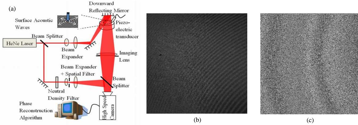
Fig. 1 (a) Experimental Setup (b) Example of interferogram and (c) the corresponding phase reconstruction.
