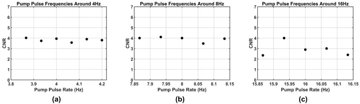
Supplemental Fig. 4. CNR measurements vs. peristaltic pump pulse frequency in the neighborhoods of three harmonics of the 2 Hz magnetic driving frequency. The data show that CNR does not significantly decrease when the pump rate is scanned across harmonic frequencies of 4, 8, or 16 Hz.
