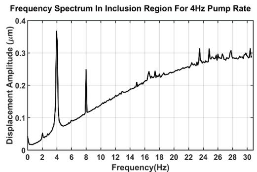
Supplemental Fig. 5. Representative B-on frequency spectrum of motion at inclusion depth, with 4 Hz peristaltic pump pulse frequency, and 2 Hz magnetic driving force. Despite the larger amplitude of displacement induced by the pump in the imaging region, the frequency and phase-locking algorithm successfully suppressed this noise, leading to a CNR of 4.0.
