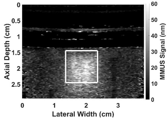
Supplemental Fig. 3. MMUS image corresponding to the frequency spectrum in Supplemental Fig. 1. This is a gelatin blood vessel-mimicking phantom with a 5 kPa elastic modulus, and a 1 ml inclusion in the presence of 275 ml/min (25 Hz) pulsatile flow. The pump-induced vibration amplitude in the inclusion region is ~1100 nm. Despite the high background motion compared to the 31 nm MMUS signal, this image demonstrates a CNR of 6.3.
